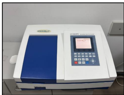
Figure 1. VWR UV-6300 PC double-beam spectrophotometer
