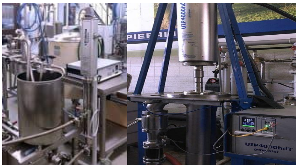
Figure 3 UIP4000hdT (4 kW) ultrasonic extraction system
