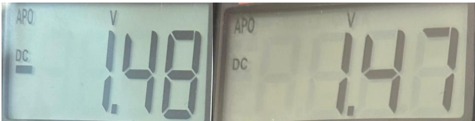
Figure 5: Observed Voltages Slightly Lower Than the Expected 1.5 V Nominal Value
