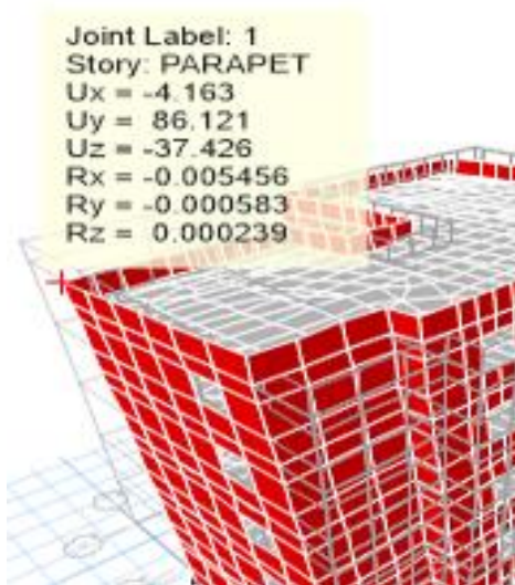
Fig. 3 – Displacements for the original building
