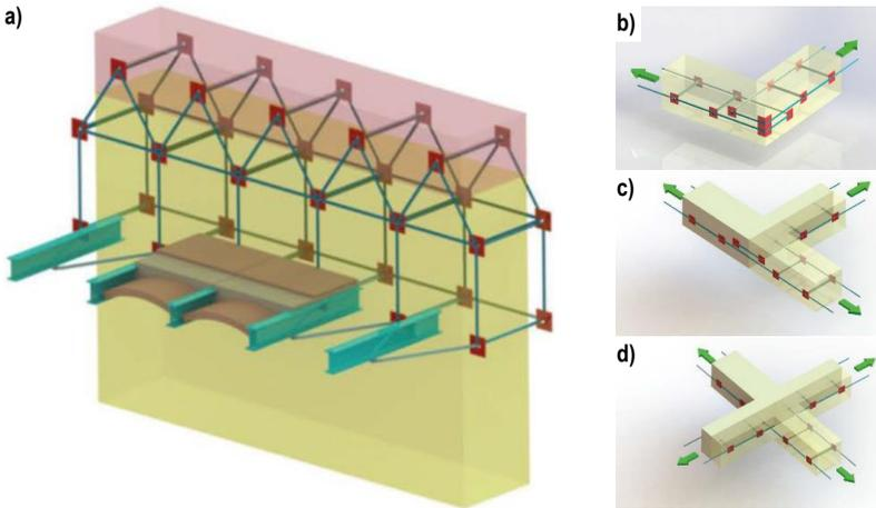
Figure 25. Connections established by the CAM ribbons between: a) the masonry wall, the upper R/C kerb and the metallic beams; b) two orthogonal walls at an external corner; c) spine and front walls in a T-shaped intersection; d) the walls of a X-shaped intersection (Marnetto et al., 2014).
