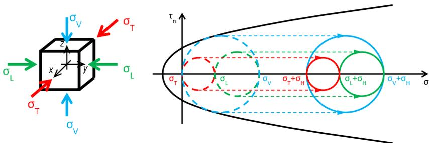
Figure 33. How the assumption of hydrostatic state of stress modifies the circles of Mohr (Mohr's circles before retrofitting in dashed lines, for comparison).
