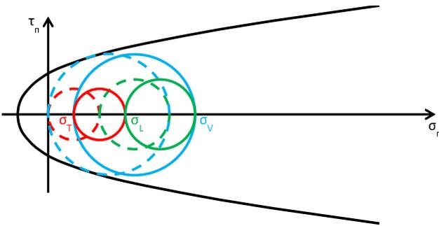
Figure 37. State of stress after the application of the CAM system for  $0 < \sigma_T \leq \sigma_L$ : assumption of hydrostatic state of stress provided by the retrofitting system (Mohr's circles before retrofitting in dashed lines, for comparison).
