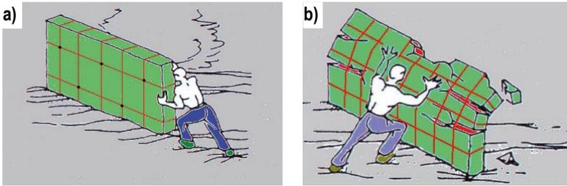
Figure 31. a) In-plane loading of a wall reinforced with the CAM system: the case of shear load (Marnetto et al., 2014); b) Out-of-plane loading of a wall reinforced with the CAM system (Marnetto et al., 2014).
