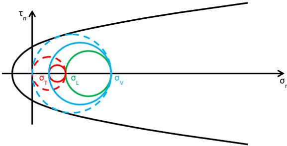
Figure 36. State of stress after the application of the CAM system for  $0 < \sigma_T \leq \sigma_L$ : assumption of perfect balancing of the in-plane forces (Mohr's circles before retrofitting in dashed lines, for comparison).
