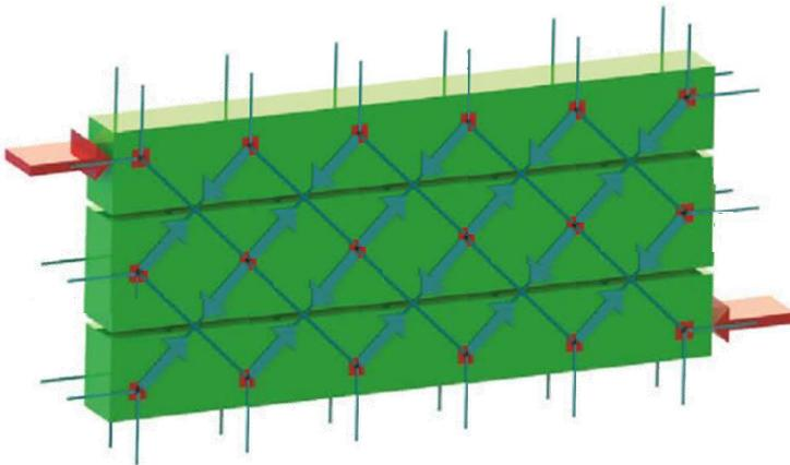
Figure 29. Optimized arrangement of ribbons for in-plane shear loads.
