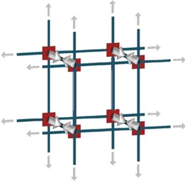
Figure 35. Mechanism of stress transfer in the assumption of perfect balancing of the in-plane forces: the thick arrows represent forces transmitted to the masonry, while the thin arrows represent forces on the ribbons.
