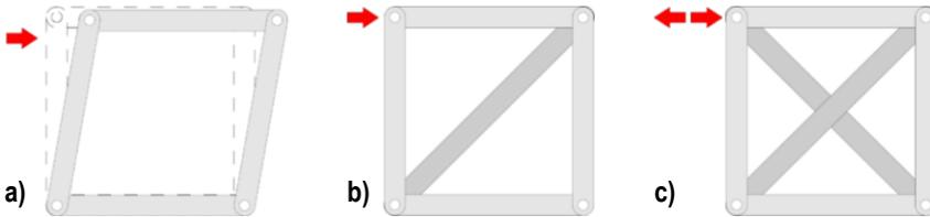
Figure 27. a) A rectangle made of hinged strips collapses when we apply a force to the side; b) By adding a strip along a diagonal will stop the collapse of the rectangle in one direction but not the other, as, having no resistance to bending, the diagonal strip works well as a tie but cannot be a strut; c) By adding strips along both diagonals, the rectangle will stop collapsing in both directions.
