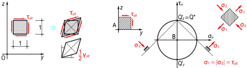
Figure 28. Deformed configuration of a plane square element subjected to pure shear in its plane: determination of the principal directions of stress in the plane of Mohr.
