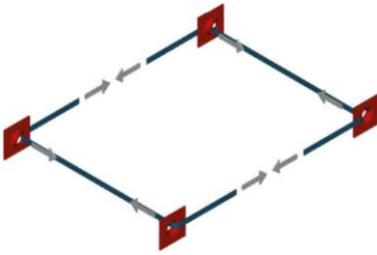
Figure 24. A closed loop of the CAM reinforcement net (Marnetto et al., 2014).
