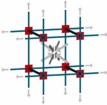
Figure 32. Assumption of hydrostatic state of stress provided by the ribbons to the masonry unit: at each corner of the unit, the resultant of the forces transmitted to the masonry is directed toward the barycenter of the unit.
