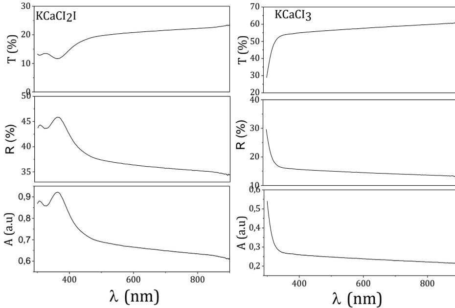
Fig. 2 The transmission, reflection, and absorption spectra of the  $\text{KCaCl}_2\text{I}$  and  $\text{KCaCl}_3$  perovskite thin films.
