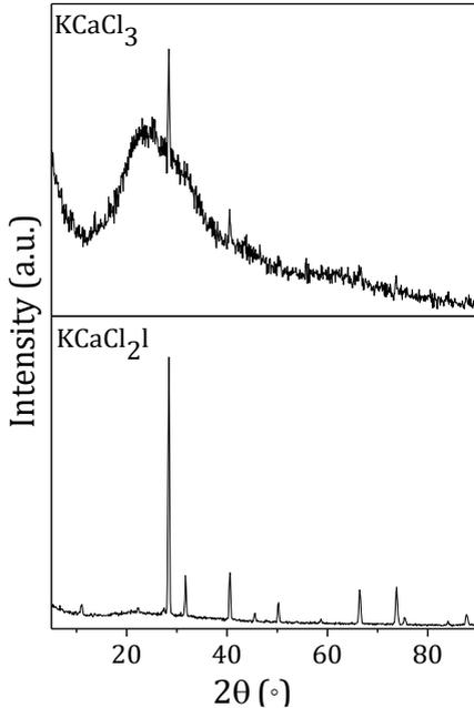
Fig. 1. XRD diffractograms pattern of KCaCl<sub>2</sub>I perovskite thin film and KCaCl<sub>3</sub> perovskite thin film.
