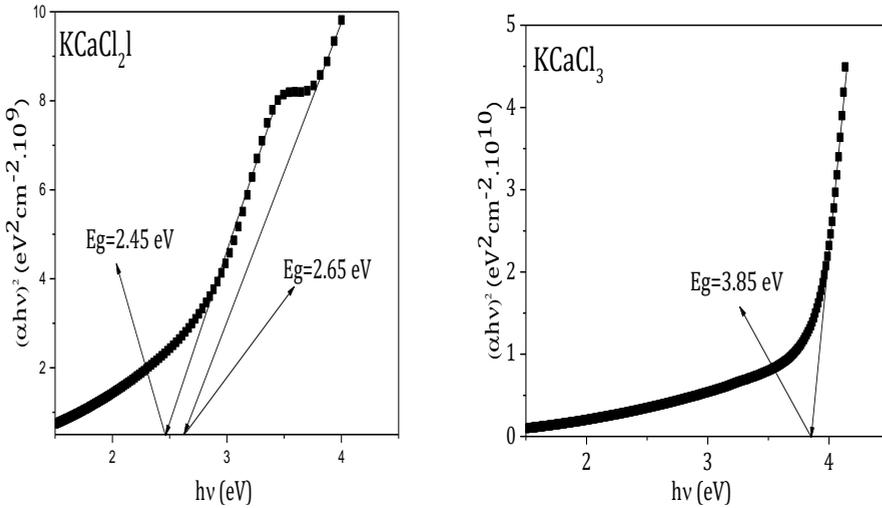
Fig. 3  $(\alpha h\nu)^2$  versus photon energy for the KCaCl<sub>2</sub>I and KCaCl<sub>3</sub> perovskite thin films.
