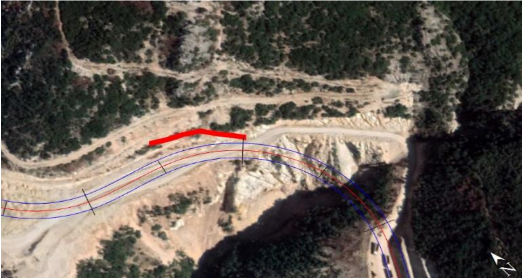
Figure 12. Rockfall barrier- km 13+550
