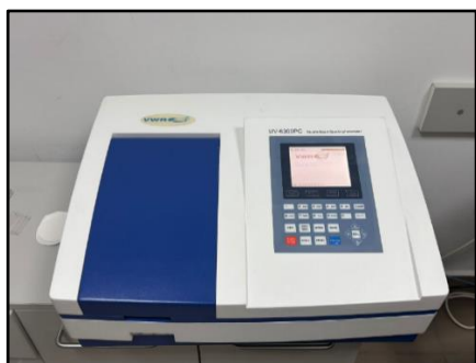
Figure 1. VWR UV-6300 PC double-beam spectrophotometer
