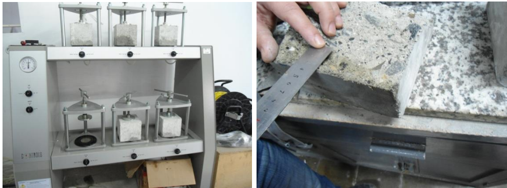
Figure 3.2.1: Images of water penetration
