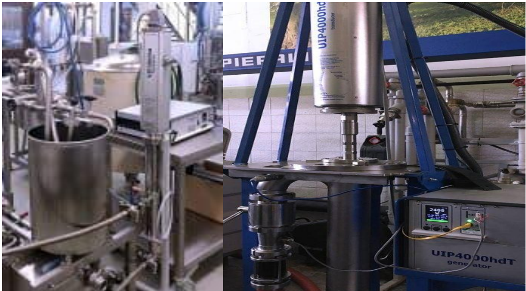
Figure 3 UIP4000hdT (4 kW) ultrasonic extraction system
