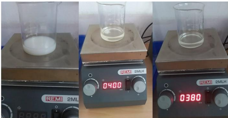
Preparation of nano Phase change material using paraffin and ZnO Nanoparticles
