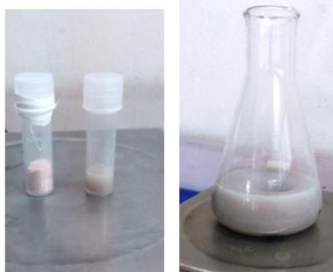
Preparation of nano Phase change material using paraffin and ZnO Nanoparticles
